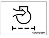
This lamp blinks when the filter of air cleaner is clogged.
