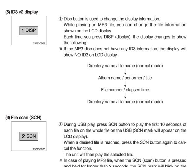
and held for longer than 2 seconds, the SCN mark will blink on the LCD display and all files in the selected directory will be introduced until the file scan mode is cancelled by pressing the SCN button again or by activating the random or repeat functions.
